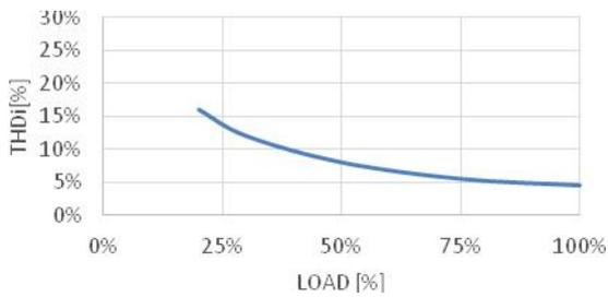
Fig. 7. THDi of input current for 160kW filter in the loading function
