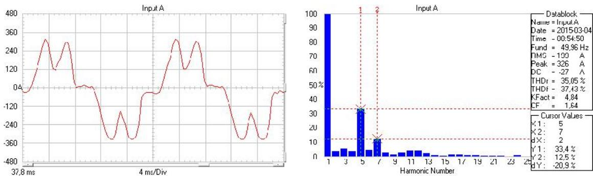
Fig. 8.b. Oscilloscope records of the input current in the converter at 5% effective impedance
