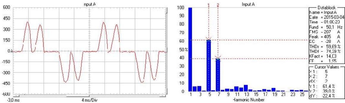
Fig. 8.a. Oscilloscope records of the input current in the converter at 1% effective impedance
