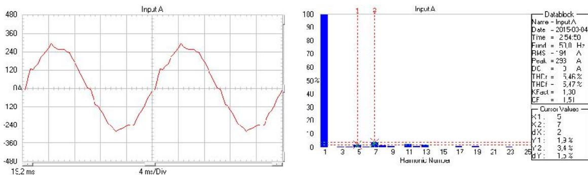
Fig. 8.c. Oscilloscope records of the input current in the converter with the harmonics filter
