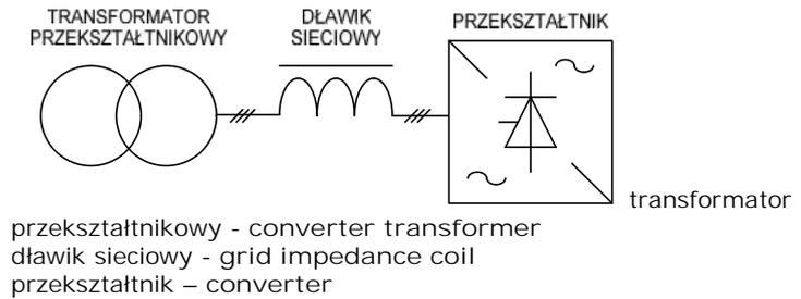
Fig. 1. Diagram of a typical converter system.
