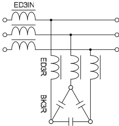
Fig. 2. Circuit diagram of ElhandHF harmonics filter
