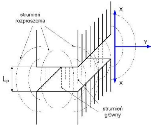
Fig. 4. Main flux and fringing flux in the by-gap area
