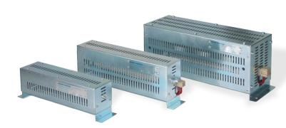
When a motor is driven by a mechanical load in the case of cranes or lifts, it acts as a generator, which converts kinetic energy into electrical energy. If there is no a regenerative system, it creates unwanted and harmful energy for the electrical motor drive system. Braking resistor, which can be connected the drive system, is therefore used to absorb this unsafe energy.
